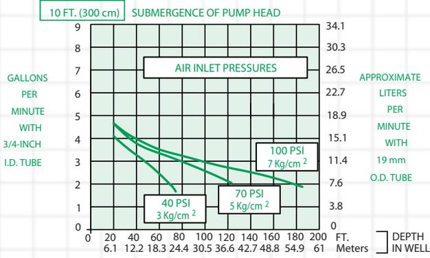
**1.00 inch (25 mm) O.D. Fluid Discharge Tubing**
