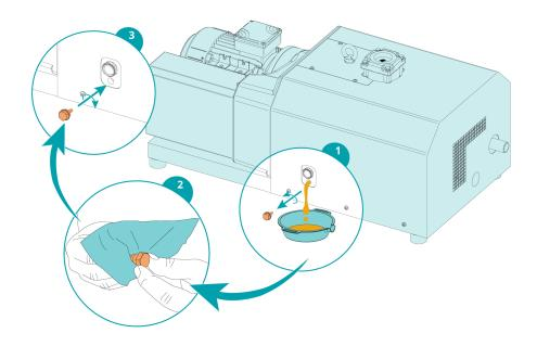
For oil type and oil capacity see *Technical Data* [ $\rightarrow$  27] and *Oil* [ $\rightarrow$  29].
