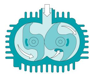
The machine works on the claw principle.
