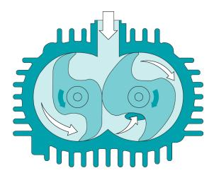
The machine works on the claw principle.
