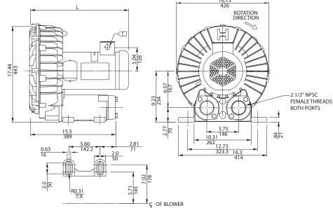
DR757CK72X 18 55/471 DR757CK86X 18.55/471 NOTES DR757D89X 18.55/471 1) TERMINAL BOX CONNECTOR HOLE 1.06 (26) DIA. DR757D86X 18.55/471 DRAWING NOT TO SCALE, CONTACT FACTORY FOR SCALE CAD DRAWING. 3 CONTACT FACTORY FOR BLOWER MODEL LENGTHS NOT SHOWN DR757D5MX 18.55/471
