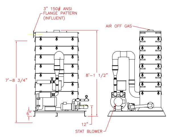
NOTE: Adjust overall height by 10 1/4" for each aeration tray added or deleted. Influent flange on the same side as effluent with odd number of trays.
