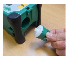
Change the filter and reassemble by turning it clockwise.
