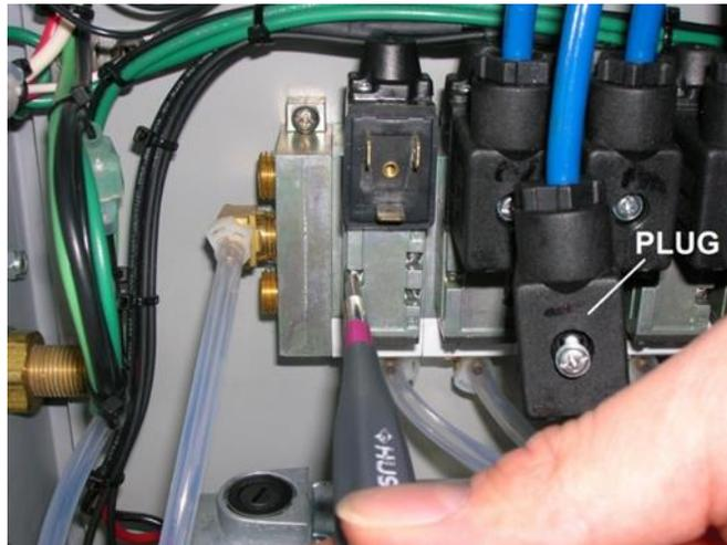
**Figure 5-1:** Removing Solenoid
