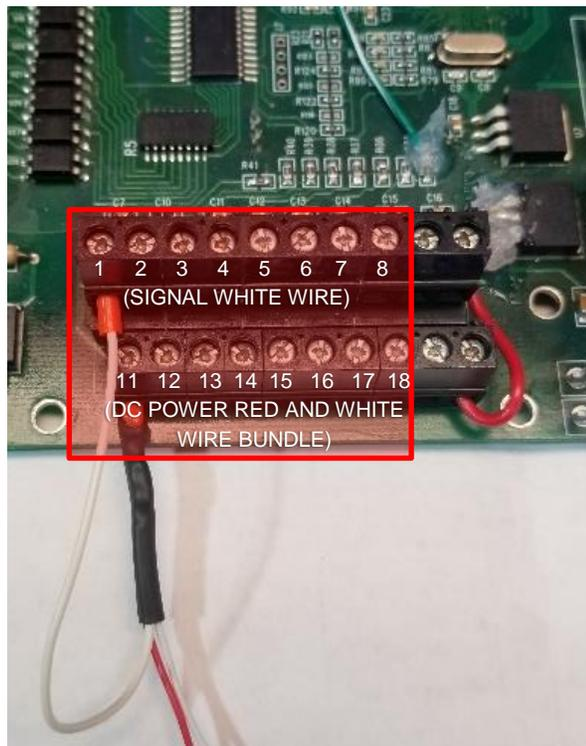
**Figure 5-10:** Additional optic sensor input DC Power/Signal
