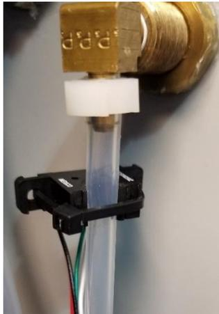
**Figure 5-13:** Optic sensor tubing installation
