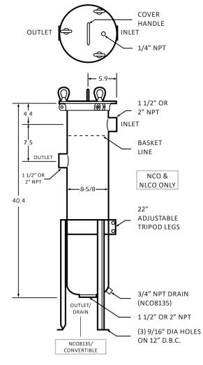
Dimensions are reference only and should not be used for hard plumbing. Consult factory for certified drawings.
