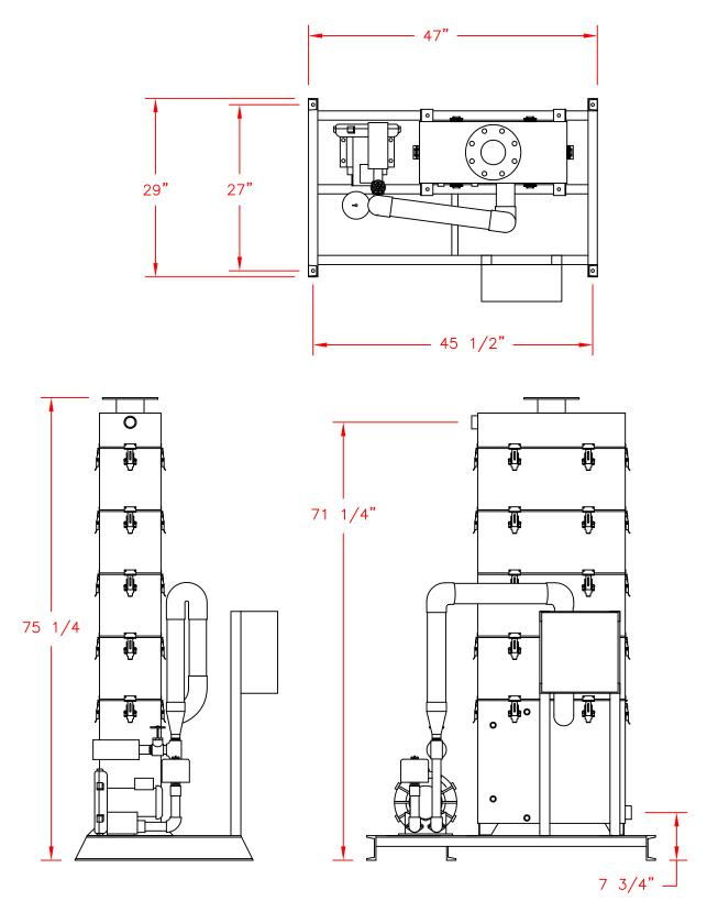
NOTE: Adjust overall height by 10 1/4" for each aeration tray added or deleted. Influent flange on the same side as effluent with odd number of trays.
