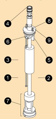
other external controls. This design allows near freezing temperature operation, reduced air consumption, and guards against unwanted adjustment or damage.
