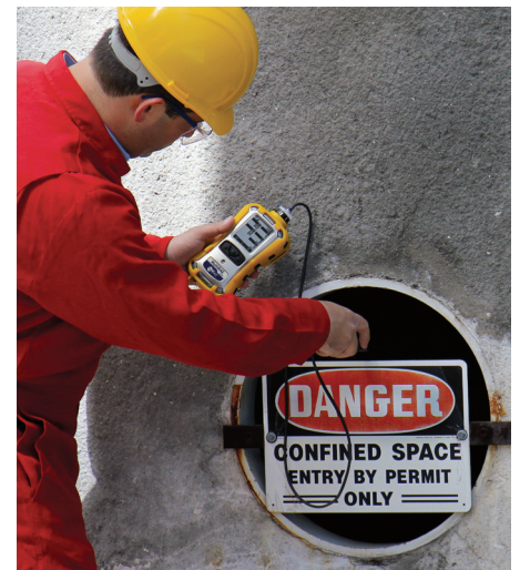
Confined space testing with the MultiRAE Lite
