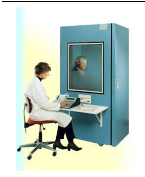
Figure 20. Testing a subject's hearing threshold levels in an audiometric booth
