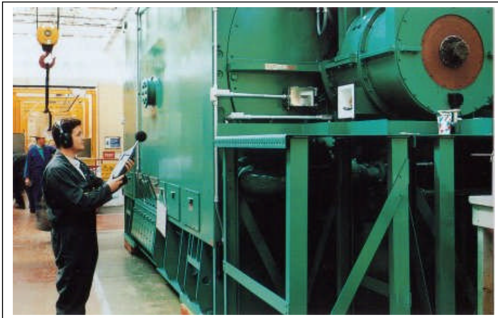
Figure 16. Collecting octave band data around a machine
