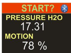
The Apex2 includes a Motion Sensor which reports a motion index expressed as the amount of time that the pump was moving. This ensures wearer compliance and confidence in the validity of the sample.
