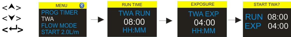
**Time weighted average (TWA)** mode allows the pump to sample for a fixed proportion of time over a specified total run time. The instrument calculates the required ON/OFF cycle to automatically spread the total sample time evenly over the entire run time (*Pro Model Only*). In this example the pump will sample for 1 minute and then pause for one minute (50:50 on off ratio) this pattern will continue for the total run duration of 8 hours.
