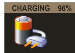
The charging display will blank after the defined display timeout period. Pressing the Power button will 'wake' the display for a further interval until timeout. Once fully charged a solid blue LED will be shown for 10 minutes, after which time, the pump will power off.
