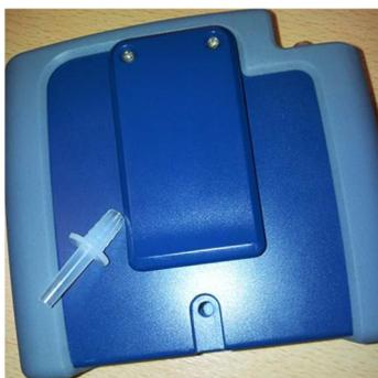
This allows the Apex2 to fill a gas bag and stop automatically when it is full.
