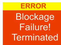
**Blockage Retry:** If the pump cannot maintain the target flow rate within 5% for more than 20 seconds (due to say a kinked tube or inlet blockage) then it will automatically halt sampling. After one minute the pump will attempt to re-start. If the specified number of retry attempts are unsuccessful, the pump will terminate the current sampling run.
