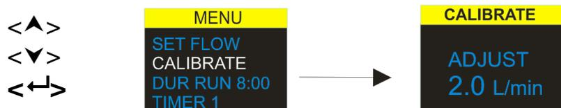
To perform a single point calibration, attach a sampling head or flow tube or other flow-measuring device to the pump's inlet nozzle then select this option to calibrate.
