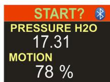
Tilt the pump forwards or backwards to automatically change the viewing angle of the display. This means you can view the display from the front whilst it is in operation and being worn by the user, or from the reverse, if you are wearing it yourself.
