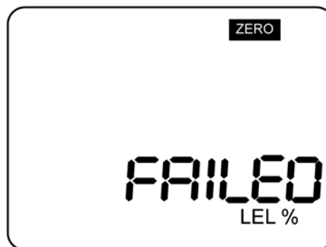
Figure 27 Zero Calibration Display - Failed
