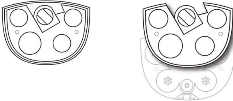
6. Turn over the plate holding the pump, and lift the pump off.
