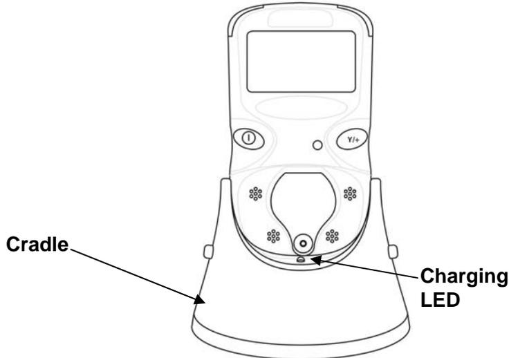
**Note:** Before setting the QRAE II into its charging cradle, visually inspect the contacts to make sure they are clean. If they are not, wipe them with a soft cloth. Do not use solvents or cleaners.
