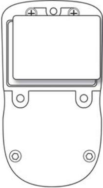
5. Place the new battery into the compartment with its six gold-plated contacts aligned over the six pins.
