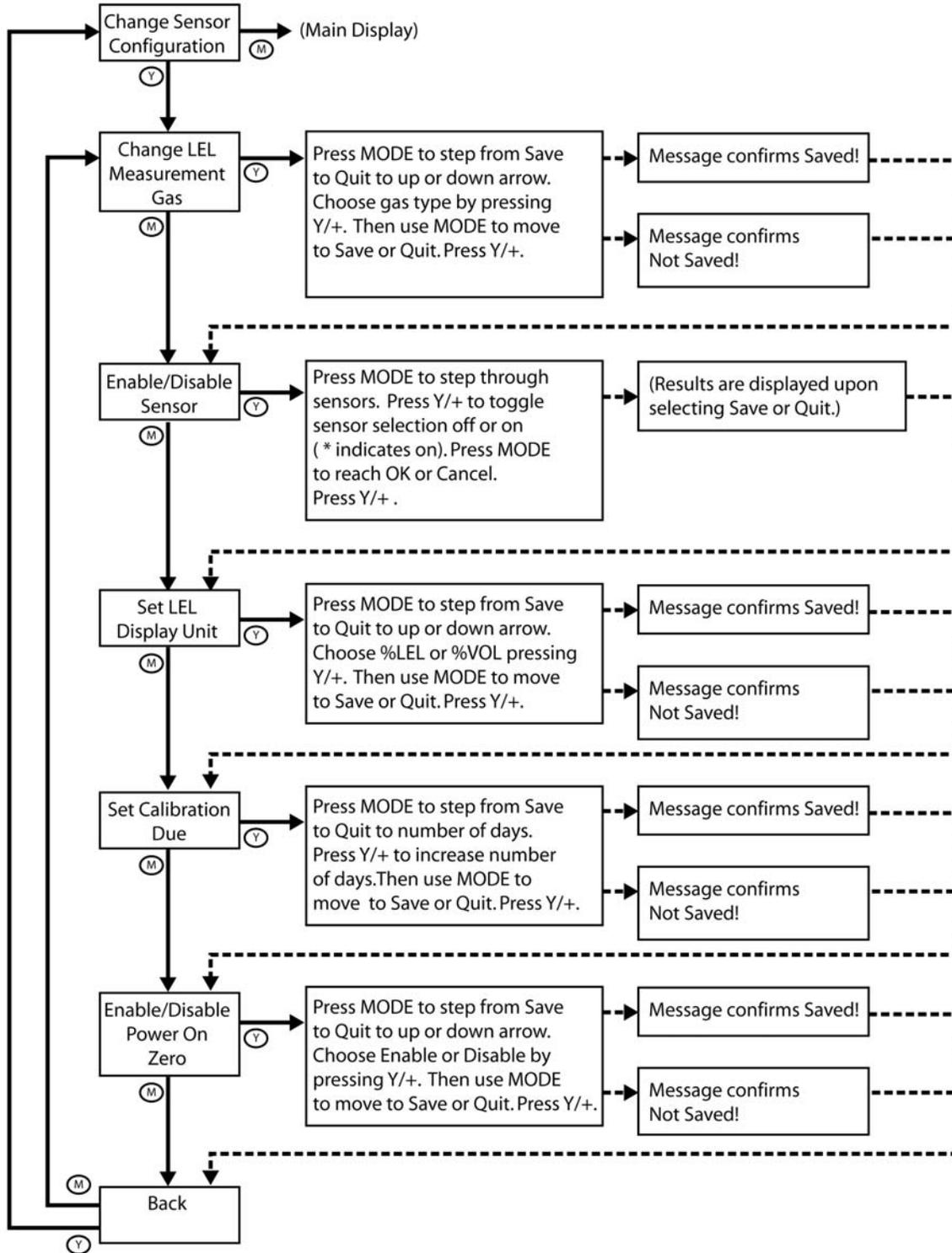
**Change LEL Measurement Gas.** This function allows selection of the measurement gas for the LEL sensor. The correction for the measurement gas is automatically divided by the correction factor the span gas, selected previously, to obtain a new factor for the combination of gases. The new factor is applied to the readings to obtain a true concentration.
