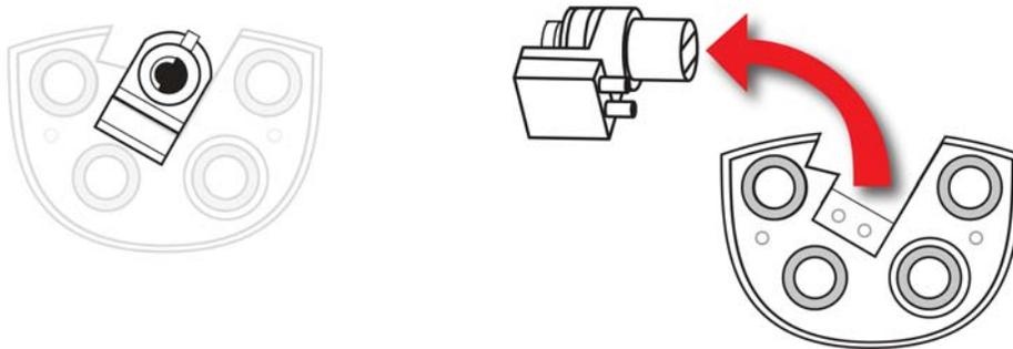
7. Replace the pump by pressing the new pump firmly into its recessed area on the plate.
