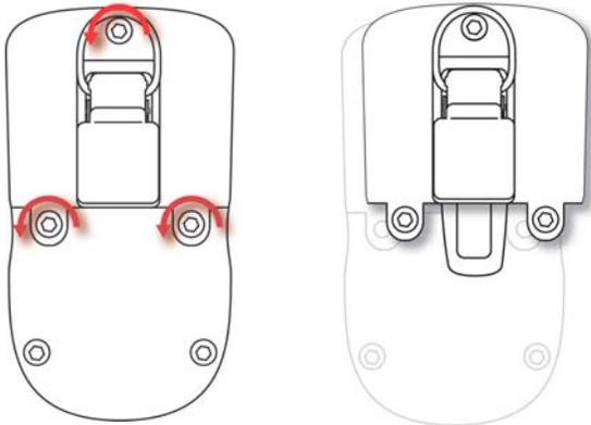
3. Hold the QRAE II down and lift the compartment cover by pulling on the belt clip.
