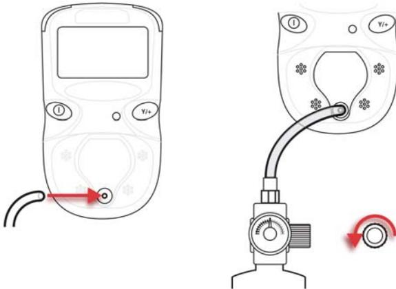
3. After calibration, turn off the gas and remove the hose from the QRAE II Pump.
