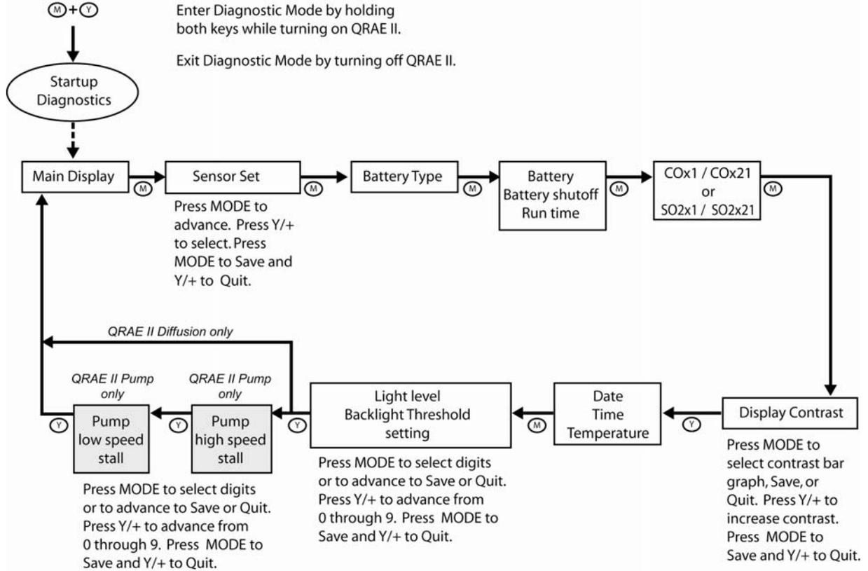
**Sensor Set.** Four sensor/sensitivity options are possible. The upper right sensor slot can accommodate either a CO sensor or an SO<sub>2</sub> sensor. The upper left sensor slot can accommodate either an H<sub>2</sub>S 0.1-100 ppm sensor or an H<sub>2</sub>S 3-1000 ppm sensor. When any sensor is exchanged for another type or value, the firmware must be set to match the sensor.
