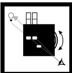
**9.** Rotate the color disc until the color matches in the two openings.
