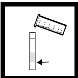
**6.** Fill another viewing tube to the first (5-mL) mark with the prepared sample.
