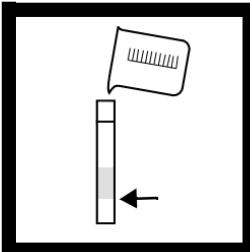
1. Fill a viewing tube to the first (5-mL) line with sample water. This is the blank.
