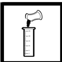
4. Add the contents of one Ferrous Iron Reagent Powder Pillow to the measuring vial.
