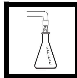
**4.** Collect a water sample directly into the titration flask by filling to the appropriate mark.
