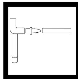
**4.** Attach a vacuum hose to the water aspirator and turn on water.
