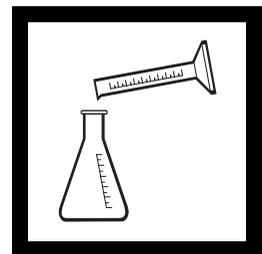
4. Use a graduated cylinder or pipet to measure the sample volume from Table 2. Transfer the sample into a clean 250-mL Erlenmeyer flask. Dilute to about the 100-mL mark with deionized water, if necessary.
