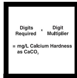
**8.** Calculate the sample concentration of calcium hardness by using one of the formulas below:
