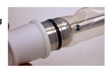
Remove the upper Teflon™ compression ring #21150042 and slide the ring off of the end of the internal tube weldment assembly #21150039. Slide the bladder #21150054 off of the internal center tube weldment assembly #21150039, at this point the O-ring #11150049 on the upper end can be replaced.
