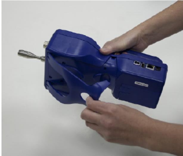
The Model 9306 is also equipped with a plastic stylus for use with the touch screen interface. The stylus locks into place in the case near the top of the unit when not in use.
