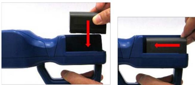
2. Place the lithium-ion battery into the battery compartment and slide it forward (toward the top of the unit) until it locks into place.
