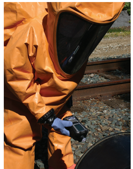
CBRN detection with the MultiRAE Pro
