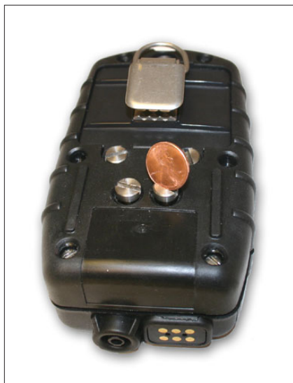
Figure 13. Loosening rear screws.
