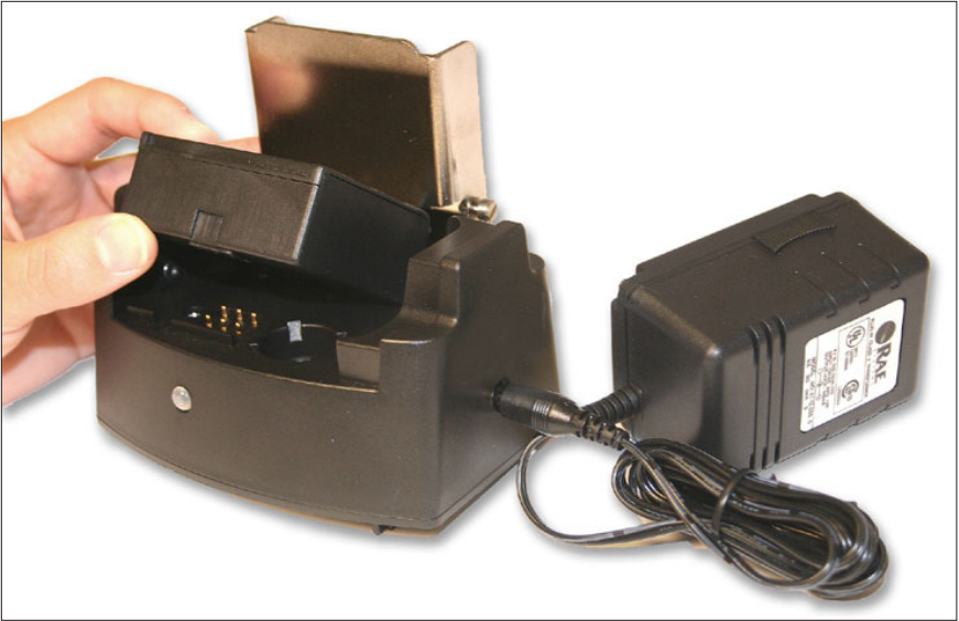
Figure 6. Installing the battery pack into the charging cradle.
