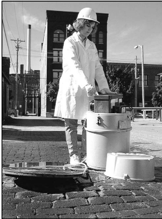
Figure 2-5 Placement of the Sampler Adjacent to Manhole
