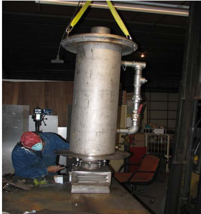
150 SCFM Catox Shell with EZ-Bolt Catalyst Module
